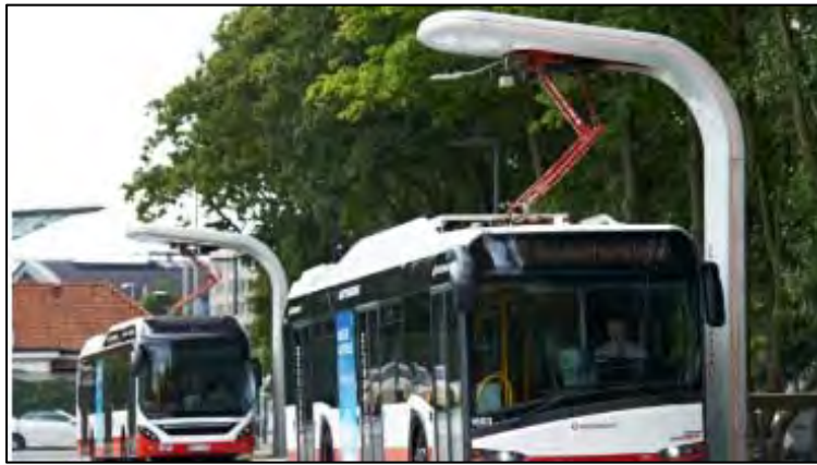
Figure 24: Bus-Down Charger (Courtesy: Siemens)
